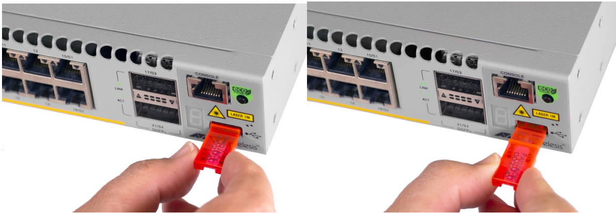
Figure 89: Removing the Housing from USB Port Lock
