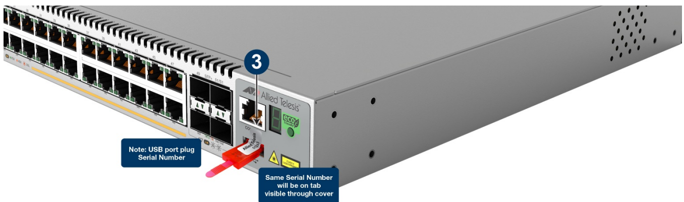
Figure 77: Location of USB Port Plug for x530L-52GTX
