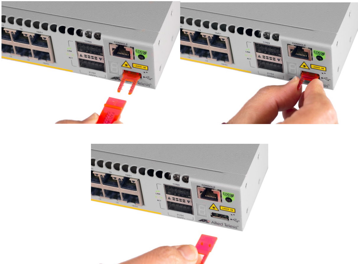
Figure 90: Removing the Last Section of USB Port Lock
