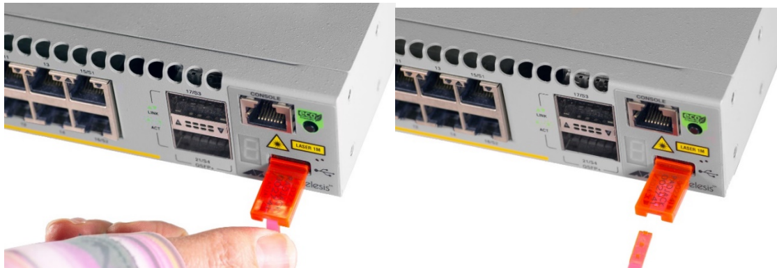
Figure 88: Breaking the Tab on USB Port Lock
