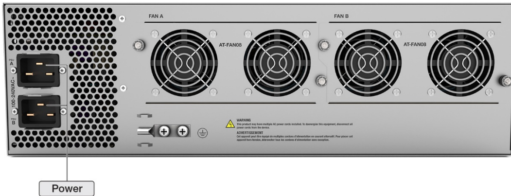
Figure 16: Interfaces on Back of AT-SBx908 Gen2
