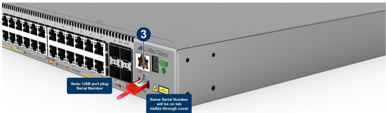
Figure 83: Location of USB Port Plug for x530L-28GPX
