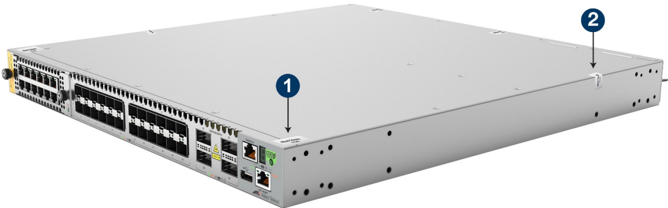
Figure 55: Tamper-Evident Seals on Top Right Side
