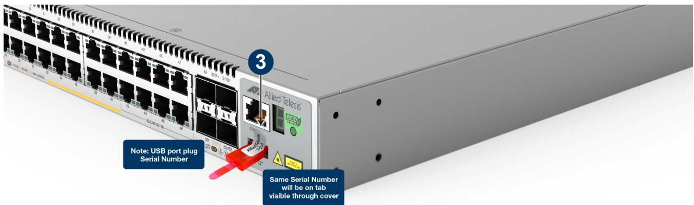
Figure 71: Location of USB Port Plug for x530-52GPXm
