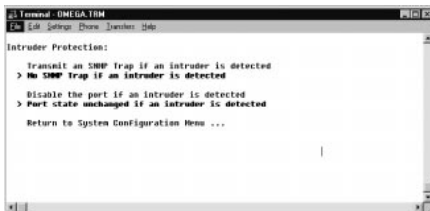
Figure 6-17 Intruder Protection Screen Section
